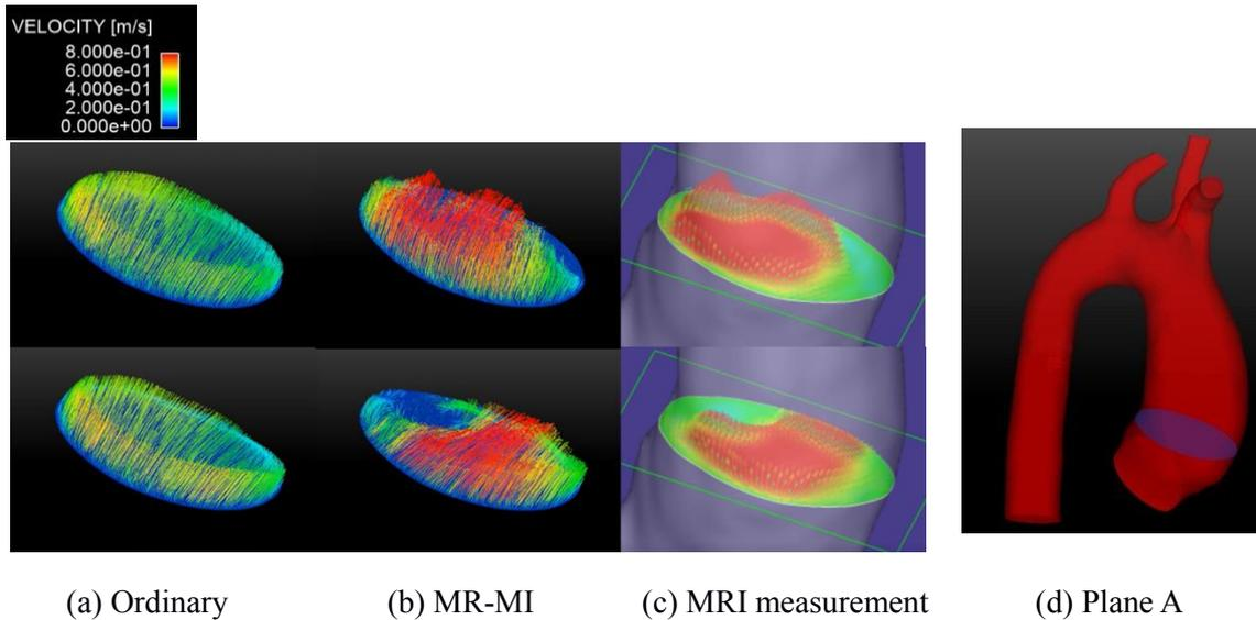
Fig. 3 Velocity profiles on Plane A colored by purple in (d). Upper and lower figures of the velocity profiles are at  $t = 0.088s$  and  $t = 0.160s$ , respectively. The same color bar for velocity magnitude is used for (a), (b), (c). The difference of the colors of the Plane A in (a), (b) and (c) is due to different visualization softwares for the numerical simulation and MR data.
