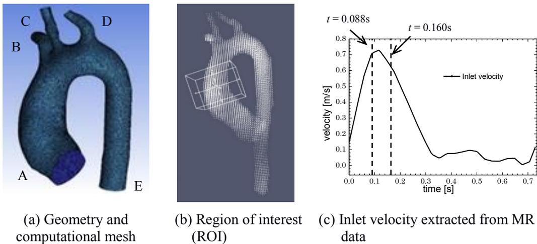
Fig.1 Geometry and computational condition
