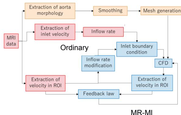
Fig. 2 Block diagram of MR-MI simulation and Ordinary simulation
